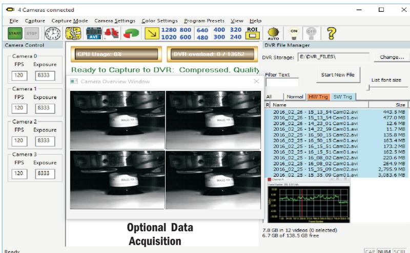
The Mega Speed MS 35K PRO camera control software is a complete software package that is included with each system. With the camera control software you can simultaneously adjust the camera settings, record the process, review the recently recorded events, edit, play back, review and transfer files without interrupting the recording process.
